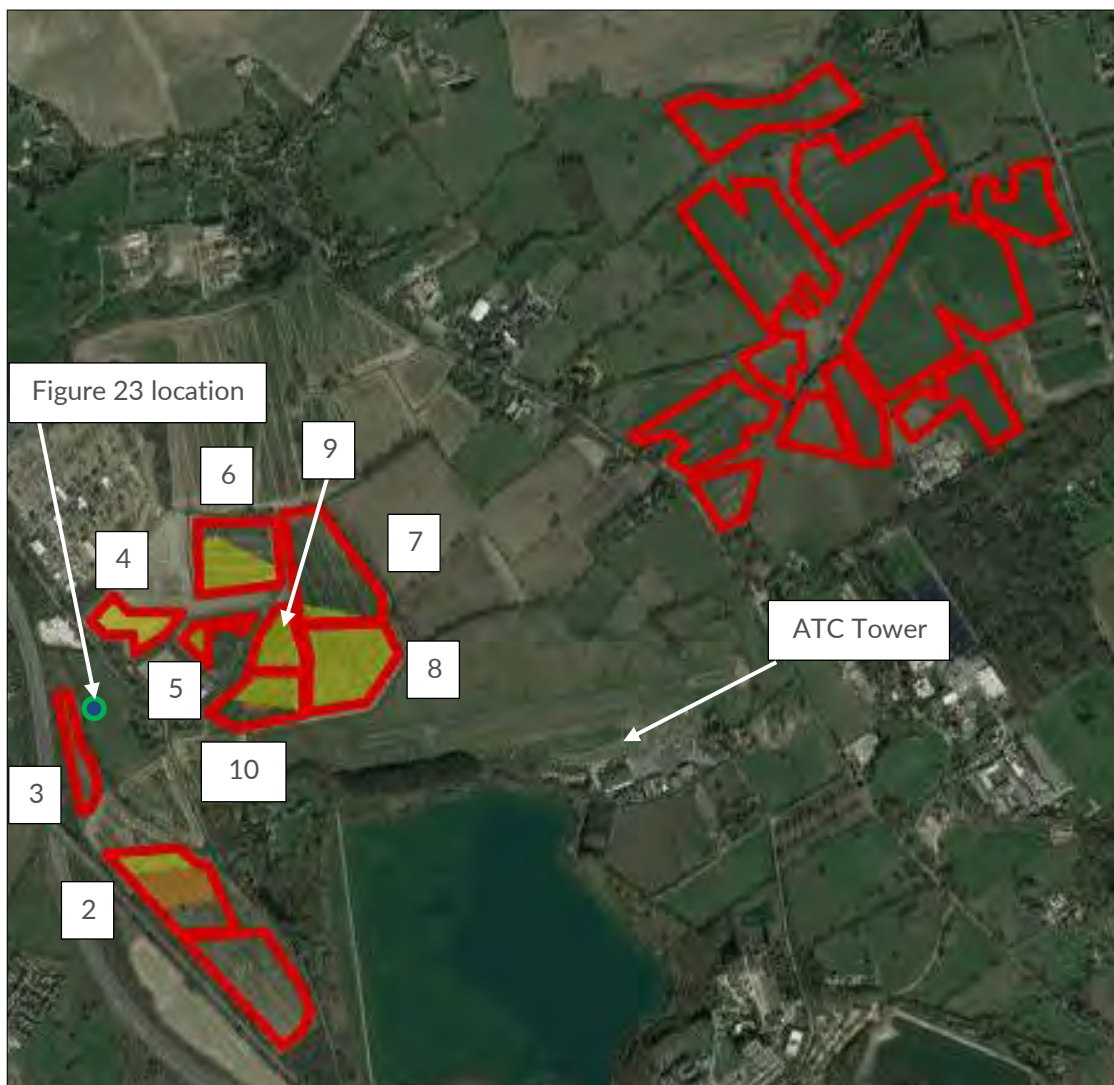
Figure 21 – Reflective areas for ATC Tower
