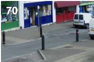
70. Well placed bollards to direct pedestrians, without over dominating the street or disrupting pedestrian flows
