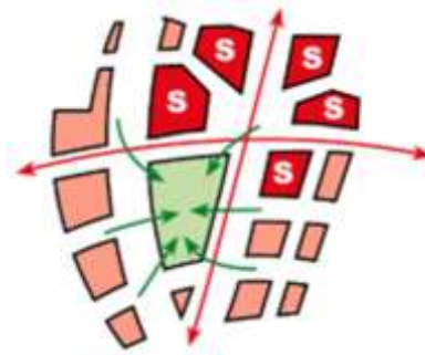
Figure 2.2: Locating services at major transport junctions and ensuring access to public spaces
