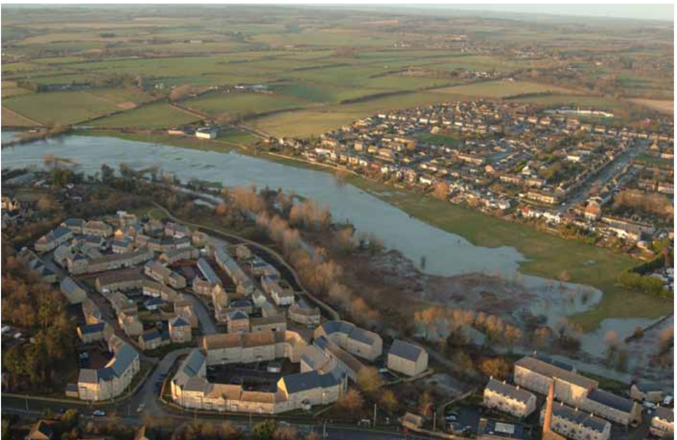
↑ New development that is set back from the river allows flooding of the natural floodplain to occur
