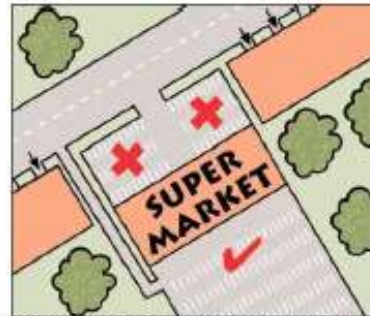
Figure 18: Access to building through area of car parking
