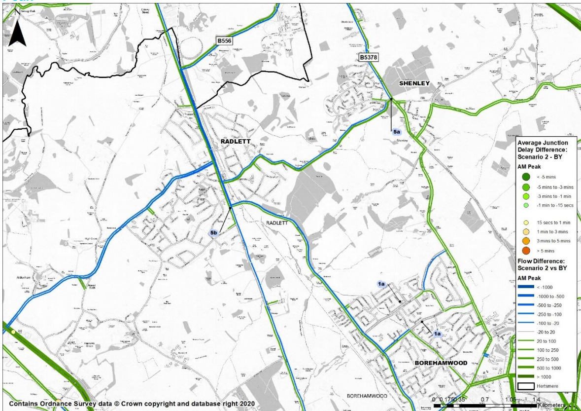
Figure 10-38: Flow and Delay difference between Scenario 2 and Base Year in Radlett - AM Peak
