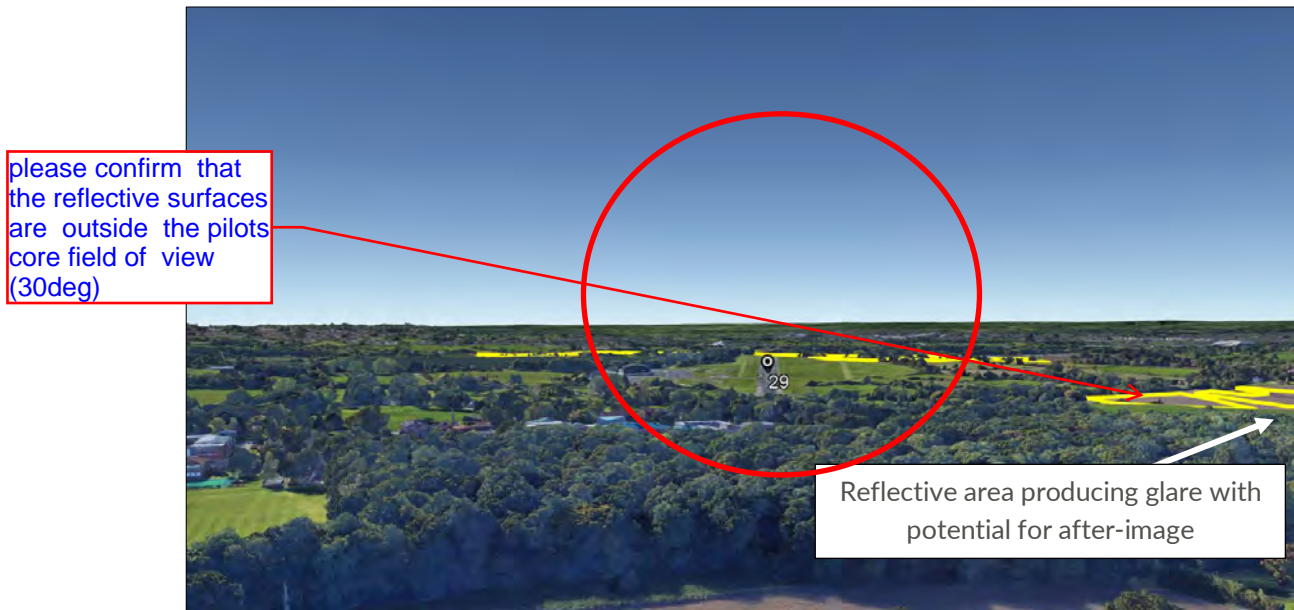
Figure 27 - View of the reflective area at 0.8 miles from the runway 26 threshold
