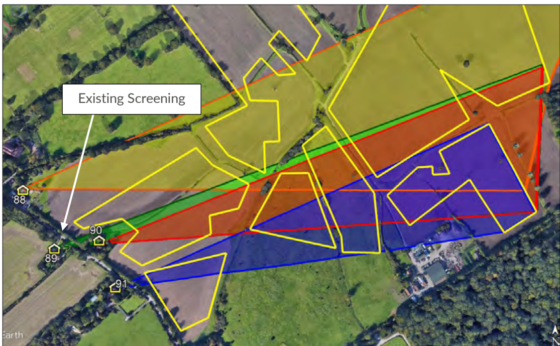
Figure 31 – Location of dwellings 88 to 91 relative to the reflective area and level of screening
