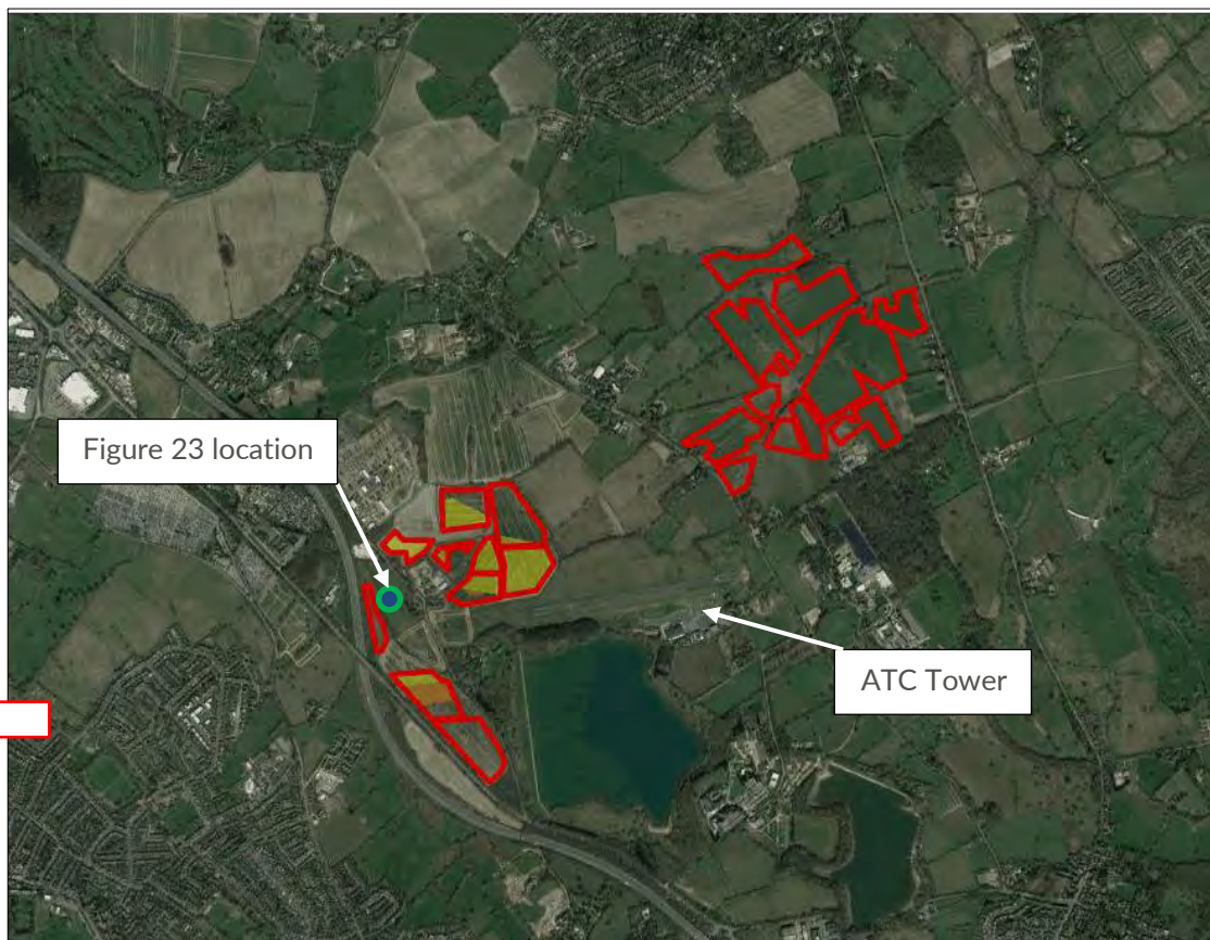
Figure 21 – Reflective areas for ATC Tower
