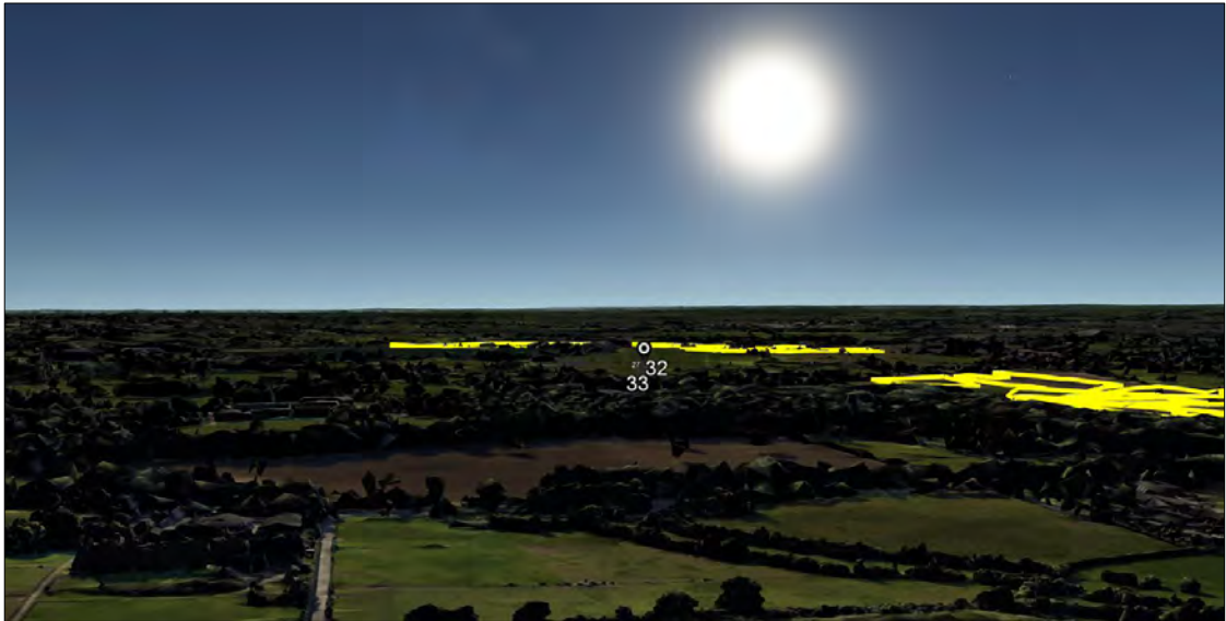
Figure 29 – Location of the sun in the sky at the time of reflection (1 st April at 17:30)
