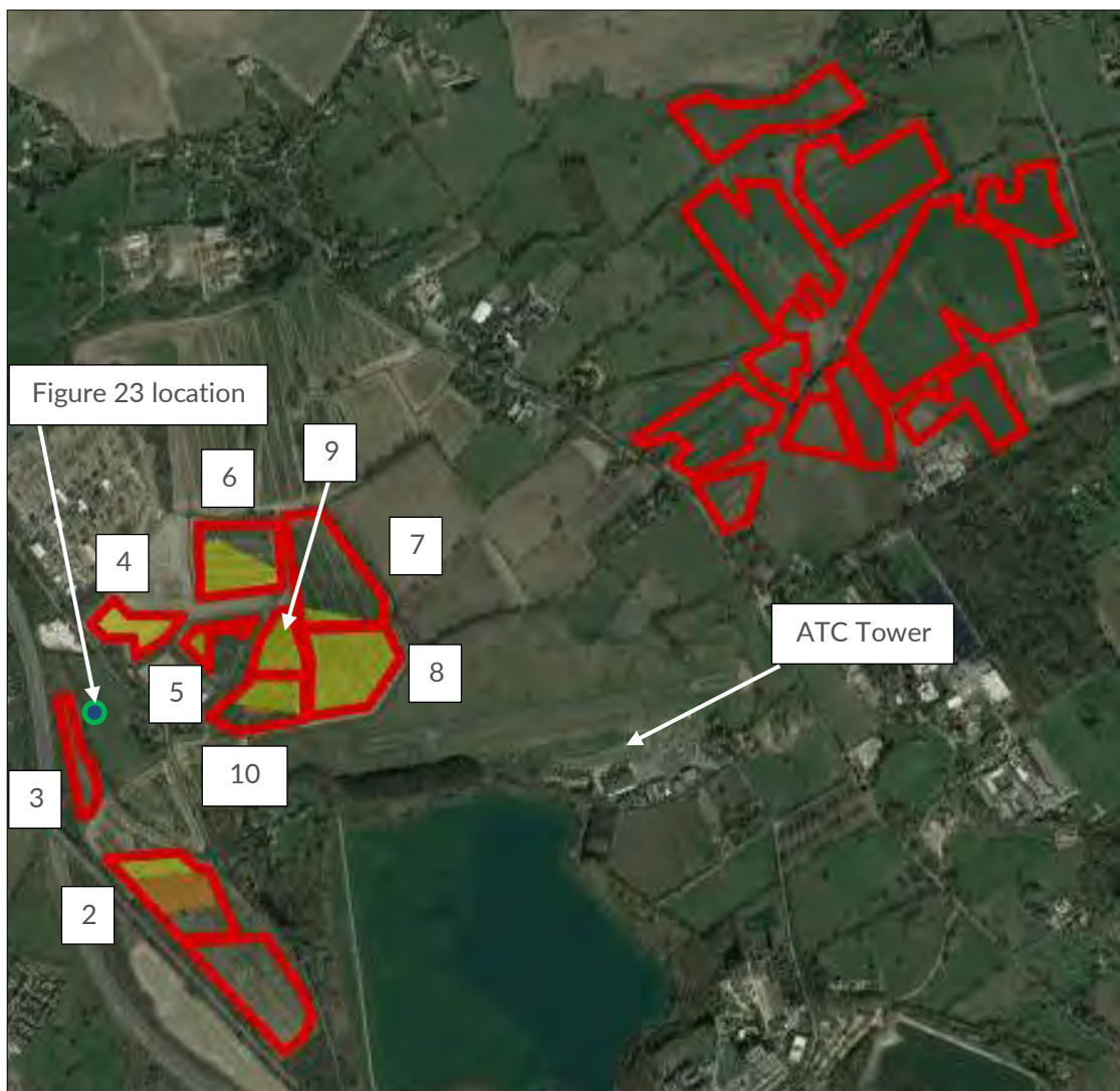
Figure 21 – Reflective areas for ATC Tower
