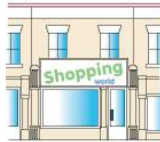
Figure 2: A disproportionate fascia board.
