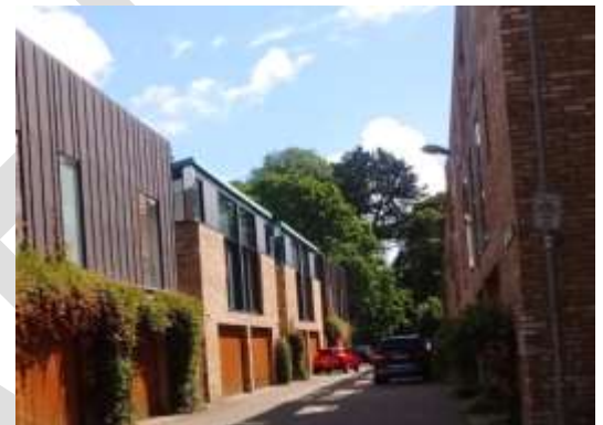
Figure 3.2: High-density development with home zones and front-to-front separation distances between 6m and 10m (Accordia in Cambridge).
