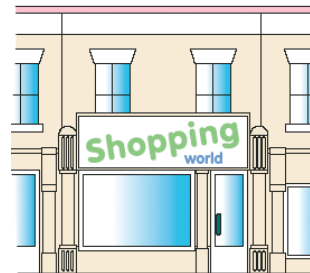
Figure 2: A disproportionate fascia board.
