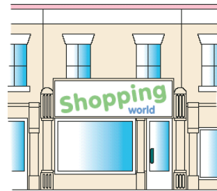
Figure 2: A disproportionate fascia board.
