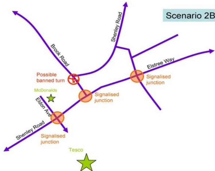
Scenario 2B_ Signalised plus bus lane in/ out of Tesco (2 lane approach on Shenley Rd west) with Banned left turn from Shenley Rd into Brook Rd
