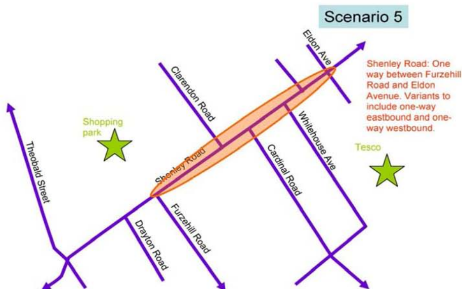
Scenario 5_ Shenley Road one way between Furzehill Road and Eldon Avenue, one-way eastbound and contra flow for buses
