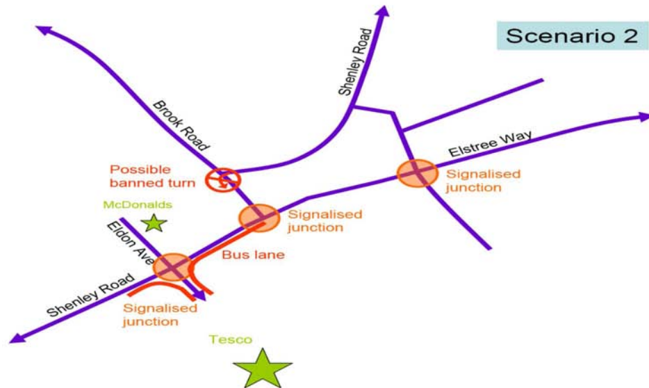
Scenario 2_ Signalised plus bus lane in/out of Tesco (one lane approach on Shenley Rd west) with no banned left turn from Shenley Rd into Brook Rd
