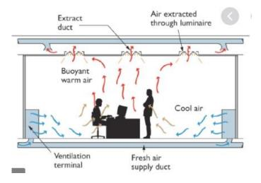
**Air conditioning** (often referred to as AC, A/C or air con) is a system used to cool down the temperature in an inside space by removing the existing heat and moisture from the room.
