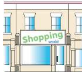
Figure 2: A disproportionate fascia board.
