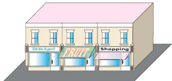
Figure 6: An example of an unacceptable blind (centre unit) and an acceptable blind (right hand unit)
