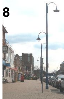
8. Good example of orderly placement lighting columns near the kerb (in the background). Note the bad placement of a mounting pole in the foreground (Darkes Lane, Potters Bar)
